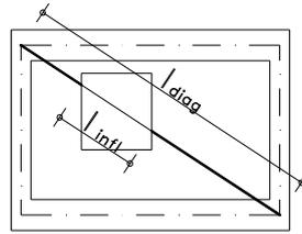
Figure 9. Equivalent strut effective length.
