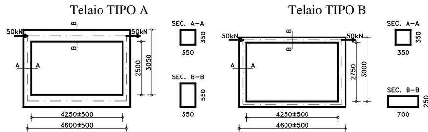
Figure 2. Frame geometry (mm).
