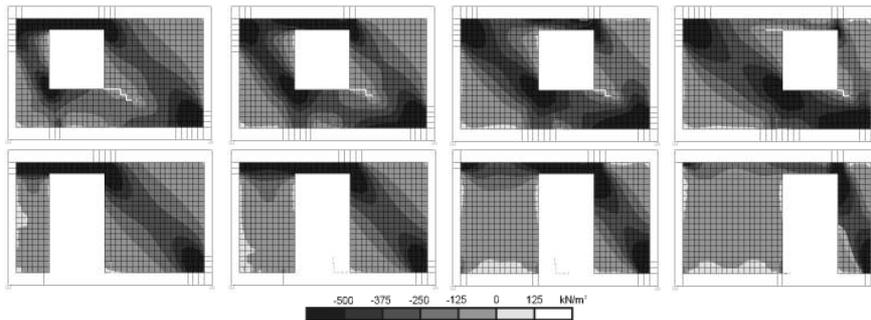
Figure 3. Frame TYPE A with window and door opening – stress distribution.
