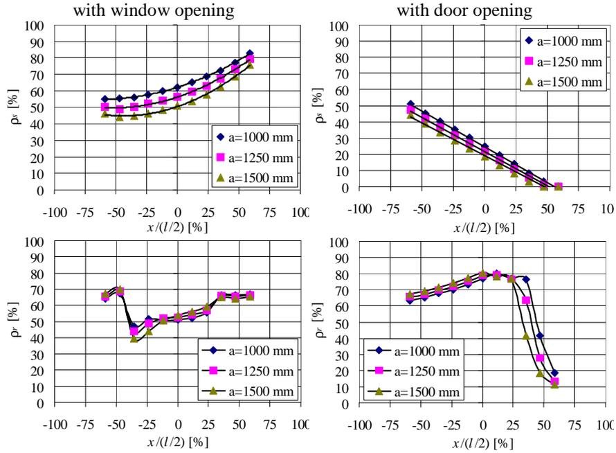
Figure 4. Frame TYPE A with window and door opening  $-\rho_s$  and  $\rho_r$  trend.
