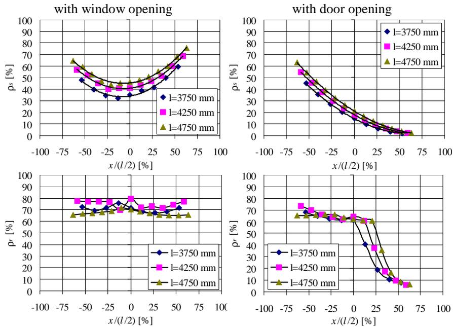
Figure 7. Frame TYPE B with window and door opening  $-\rho_s$  and  $\rho_r$  trend.
