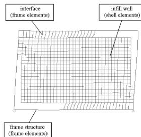
Figure 1. Proposed model scheme for infill wall.
